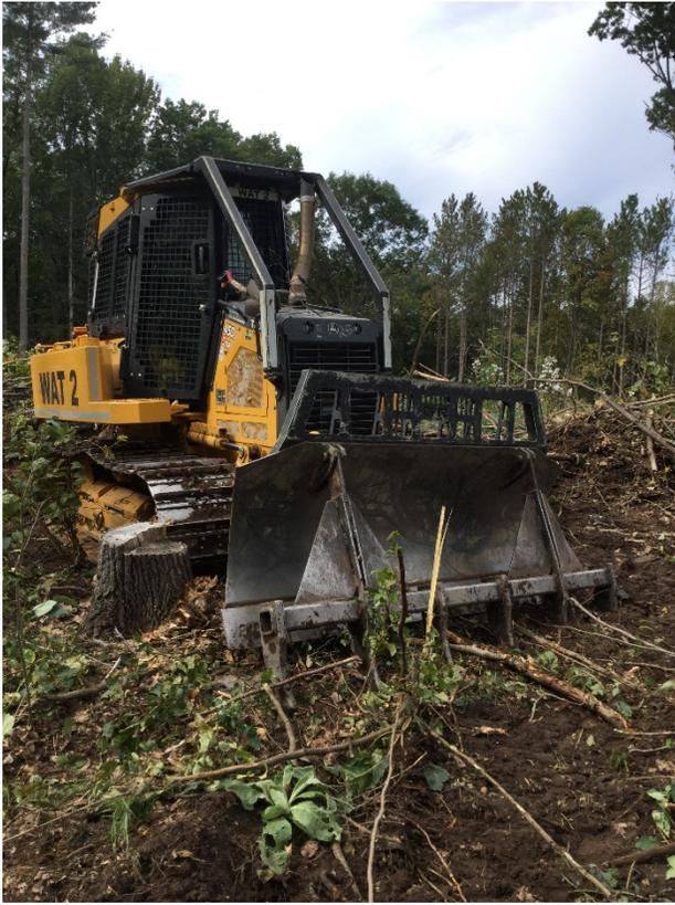
*Figure 11. A WI DNR John Deere 450 LGP with a root rake attachment*
