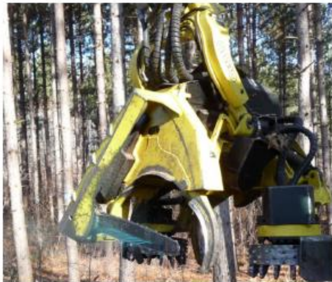
A perforated sawbar. Liquid fungicide is sprayed through small holes at the time of felling
