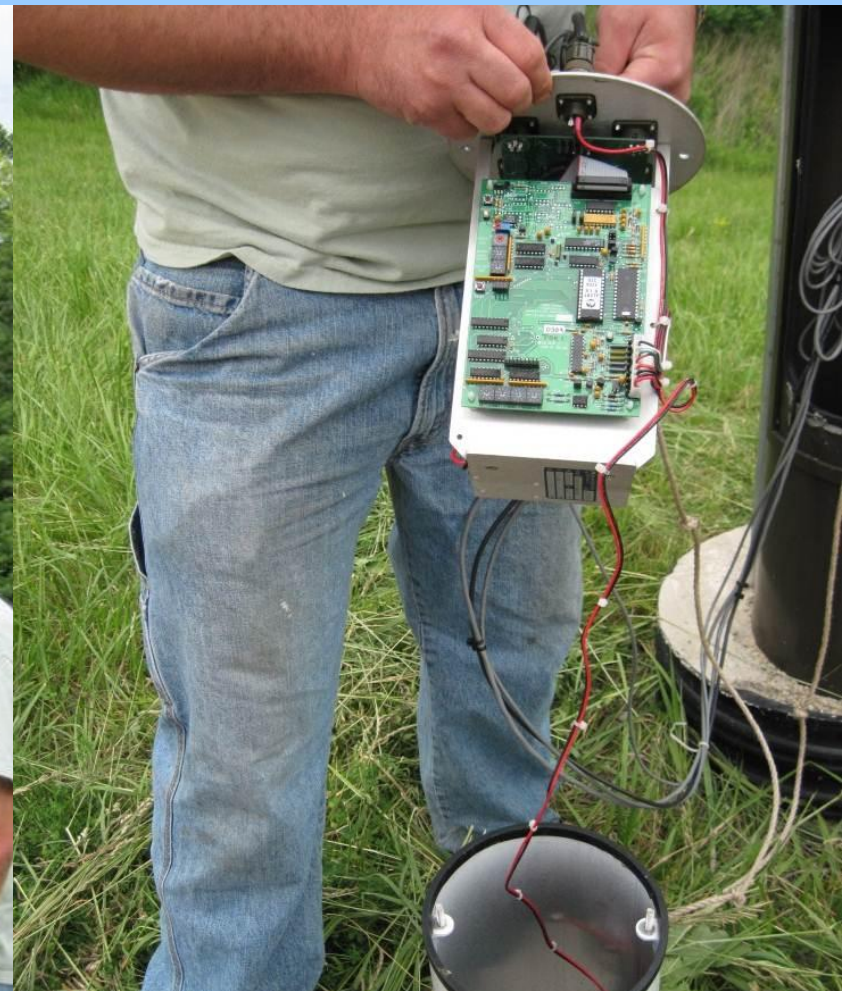
River warning systems installed on conservation dams to warn county officials about expected dam breaching.
