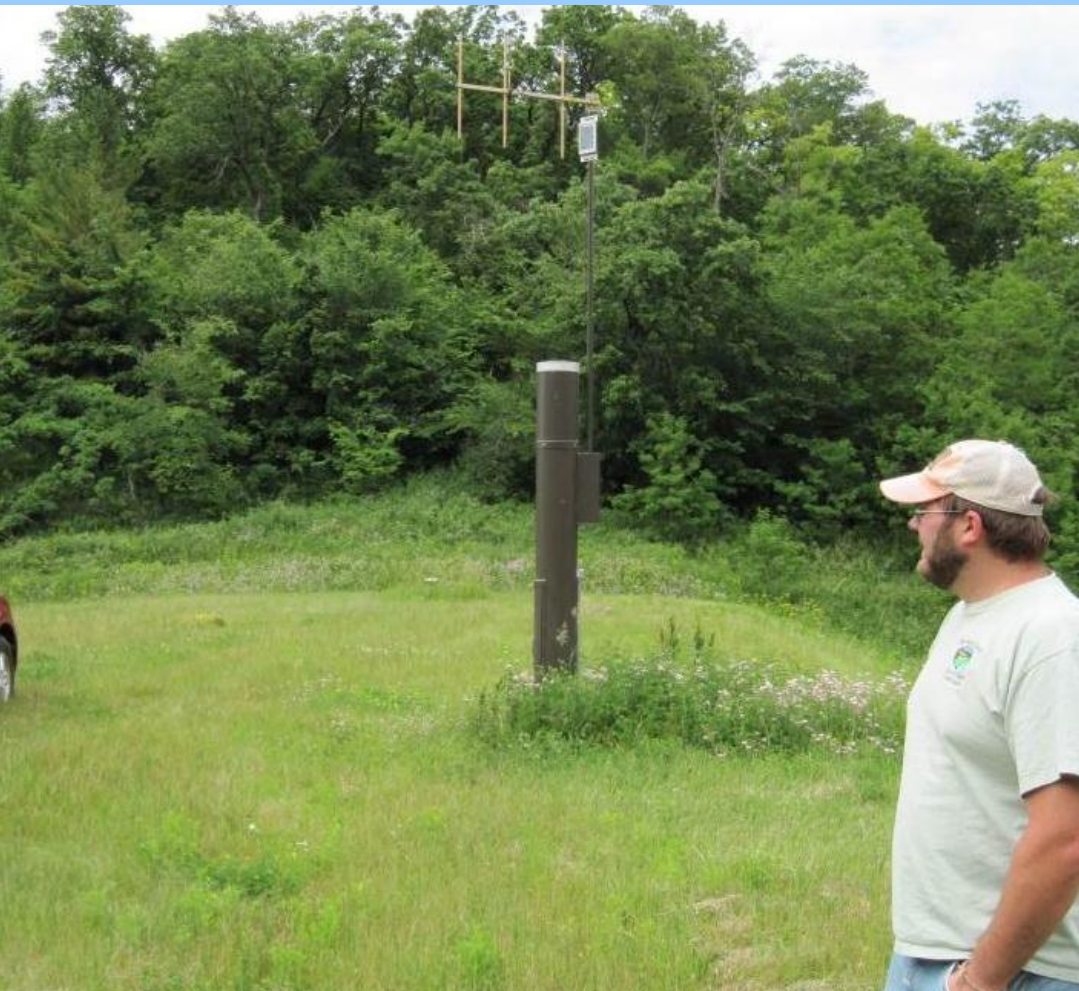
River warning systems installed on conservation dams to warn county officials about expected dam breaching.
