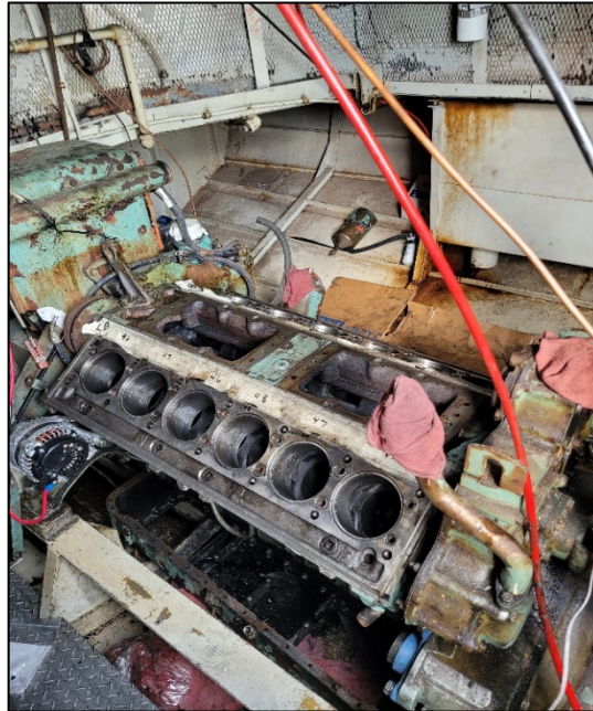
Blowers, heads, pistons, and cylinder liners removed.
