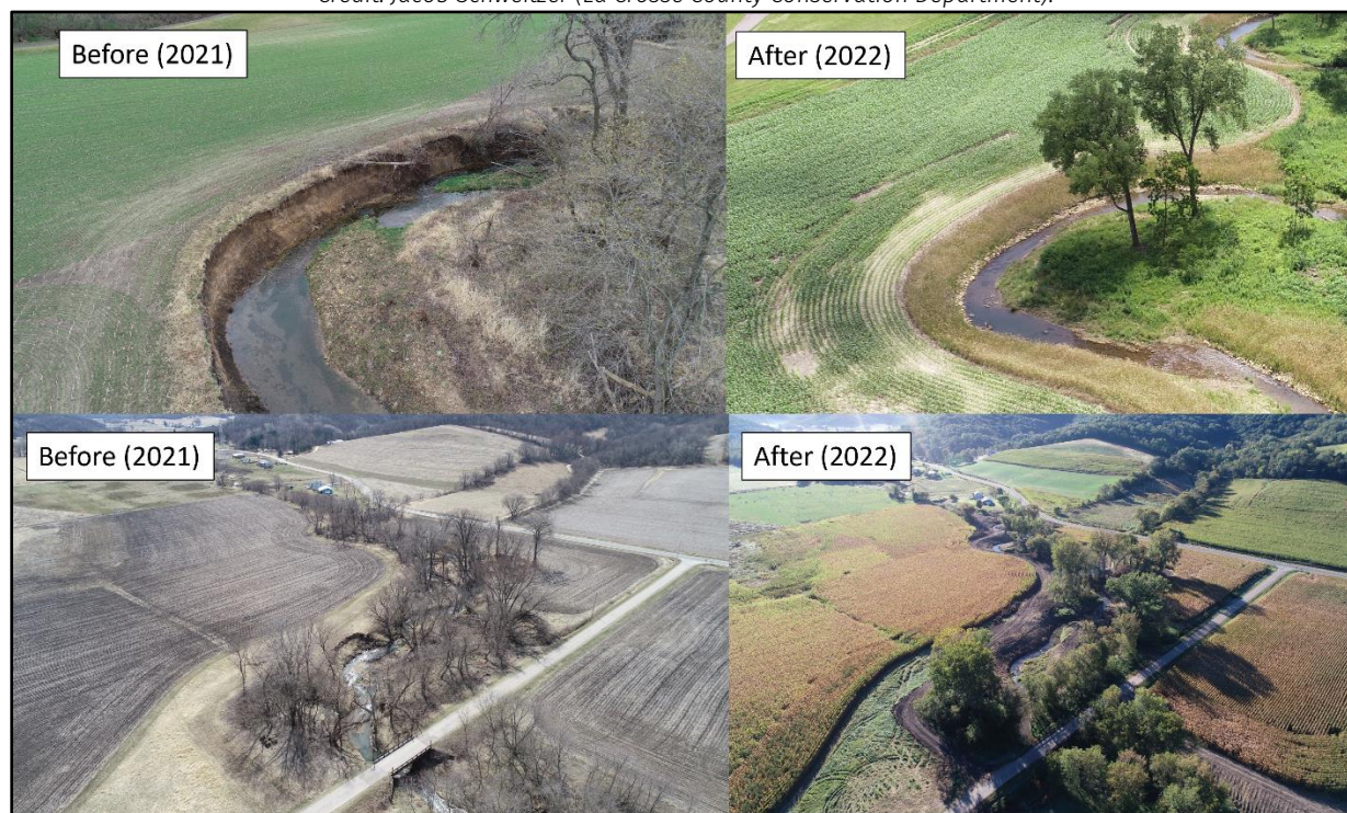
Figure 3 Bostwick Coulee Creek before and after the completion of a NRCS/La Crosse County Trout habitat and bank stabilization project in 2022. Top photos were taken upstream of Larson Coulee Rd. Lower photos were taken upstream of Drogseth Rd. Photo Credit: Jacob Schweitzer (La Crosse County Conservation Department).
