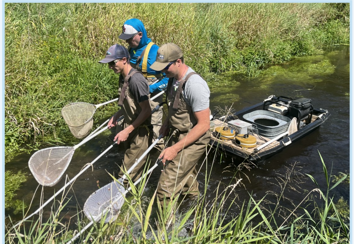
Fisheries staff sample McCann Creek in Chippewa County with a barge electrofishing unit. Fish are immobilized by electricity and then captured where biological data is collected.
