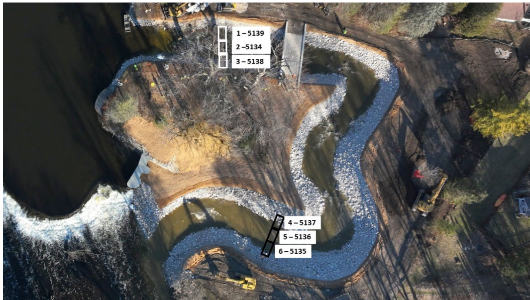
Image. Aerial photo of Kletzsch Park Fish Passage during construction. The white boxes depict the three antennas on the upstream side of the fishway and the black boxes depict the location of the downstream antennas. Photo Credit: MMS
