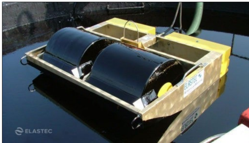
Figure 6.3-10 An oil skimmer being used to remove surface oil on water. Source: RPS Oil Spill Report- Operations Assessment Oil Spill Report, Appendix AH
