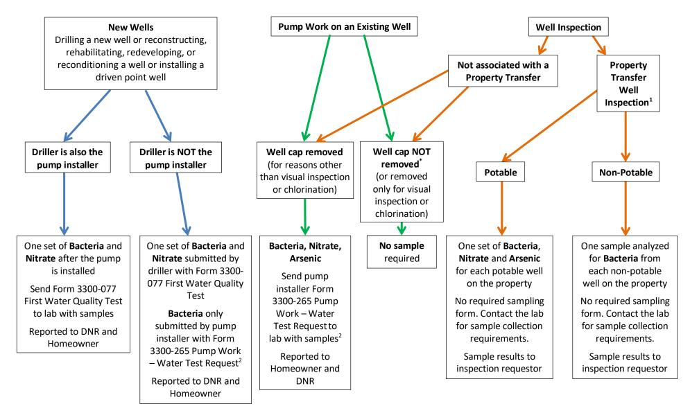
\*Opening a well cap or well seal to *visually inspect* or *chlorinate*, is not considered pump installing unless the well cap or seal is *replaced* with a different cap or seal, or unless the well has a *hand pump* installed on it. ss. NR 146.02(5) and 812.07(82). Following the measurement of a water level, collecting a water sample for coliform bacteria analysis is recommended, but not required.
