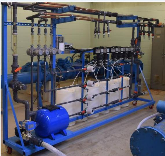
Pipe loop study underway. Harvested sections of pipe are near the top of the rack, lead toward the rear and copper in the middle.
