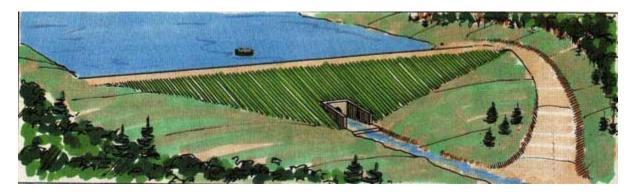
**Earth Embankment with Drop Inlet and Emergency Spillway**
