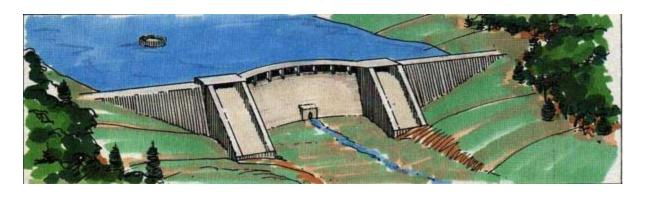
**Arch/Buttress with Pipe Outlet**
