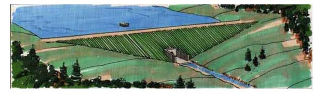
**Earth Embankment with Drop Inlet**
