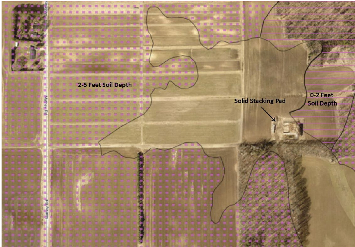
Aerial Map 4. The aerial map above illustrates mapped depth to bedrock under the satellite stacking pad. The horizontal purple lines represent 0-2 feet of soil depth to bedrock. The purple dots represent 2-5 soil depth to bedrock. The aerial image was obtained from SnapMaps.
