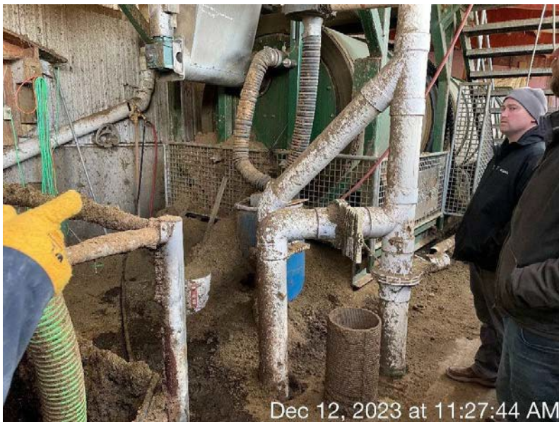
Photo 27. The solid separator that removes biosolids from the liquid manure generated in the freestall barns.
