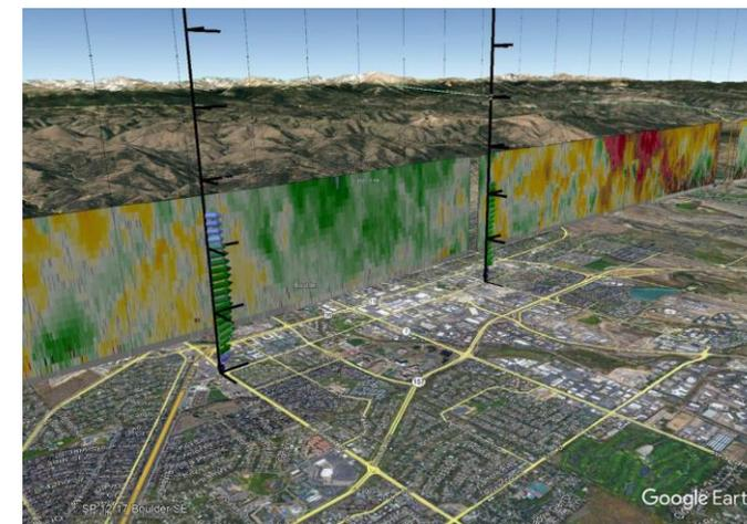
**Scanning Doppler Lidar:** Boundary layer depth and wind fields to characterize dynamics and flows over water, land and shorelines
