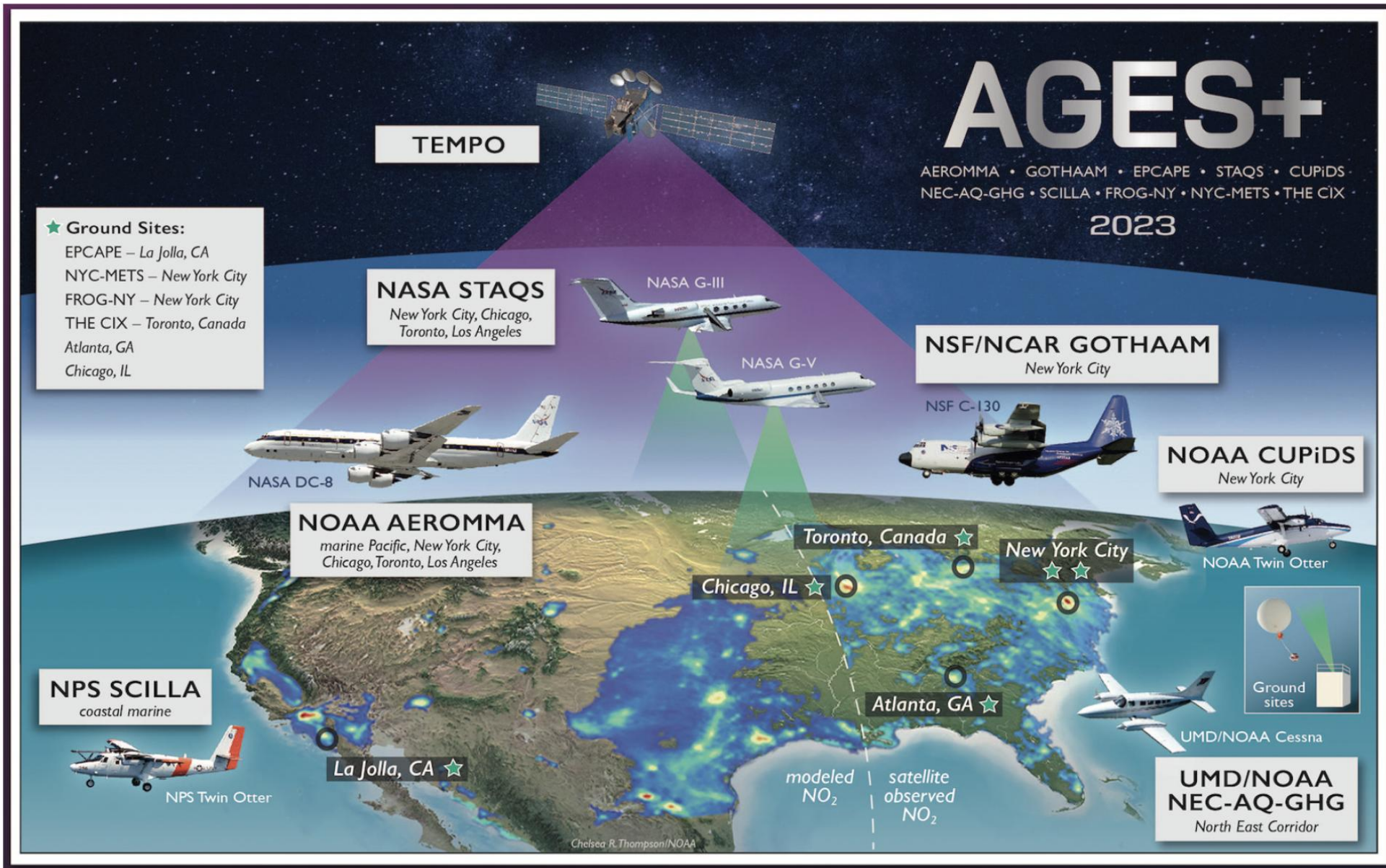
Figure 1. Example of the combined utilization of data data products to understand air quality through the set of field campaigns known as AGES+. In this schematic, satellite data from TEMPO (purple) provides a top-down estimate of NO 2 , to complement ground-based monitors, model data, and research-focused aircraft and balloon measurements (NOAA 2023).
