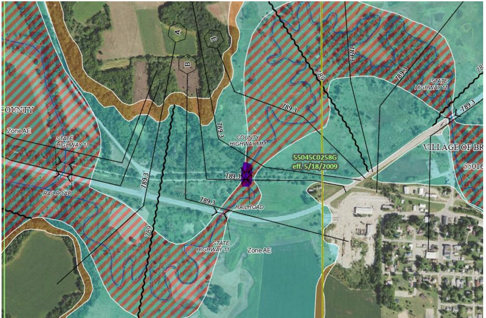
Bridge is located in the purple highlighted area. This area is within FEMA regulated floodplain.
