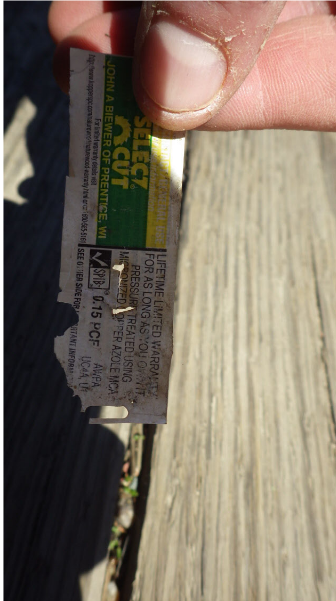
Decking is MCA treated to UC4A which is insufficient for structural applications
