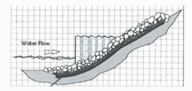
Rip-rap retainment and water flow inlet. Same on other side for water flow outlet.
