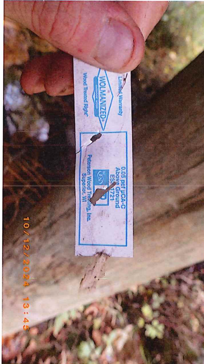
Preservative tag Copper Azole, 0.05 pcf above ground (insufficient treatment for high humidity bridge use)
